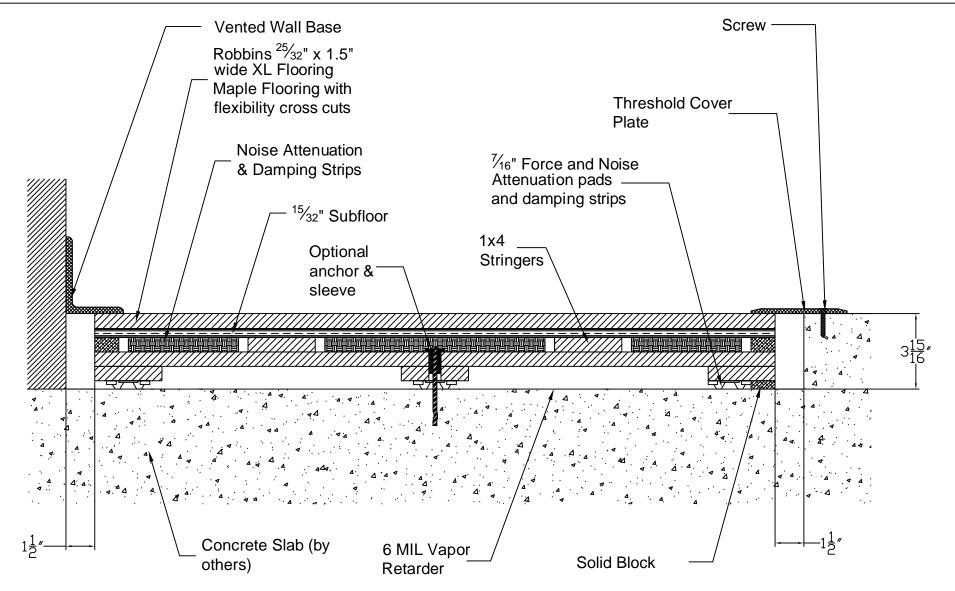
System can be installed floating or anchored.
