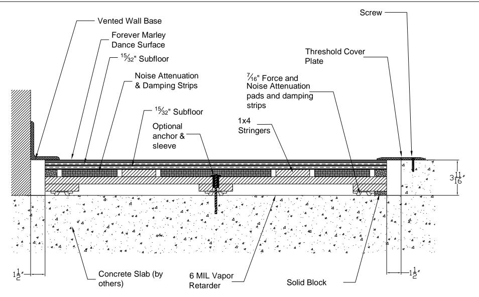
System can be installed floating or anchored.
